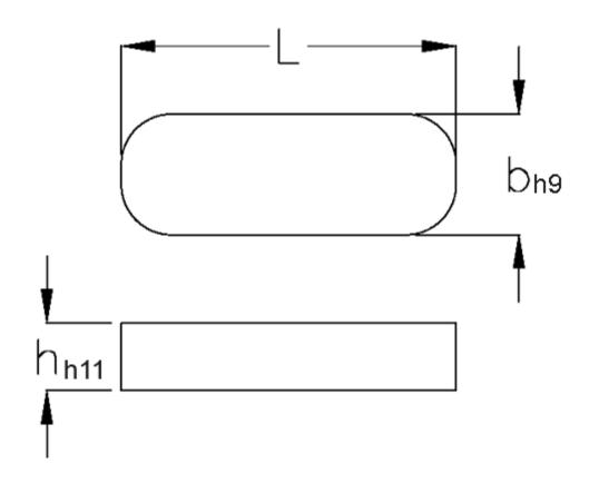
$\begin{array}{ll} b & = 16 \\ h & = 10 \\ L & = 90.0 \\ Tolerance \ b = 0.043 \\ Tolerance \ h = 0.090 \end{array}$
